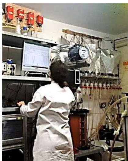
Figure 3 – Lab stand for anaerobic digestion
