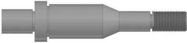
Figure 1 – Body-of-rotation type part for machining on a lathe
