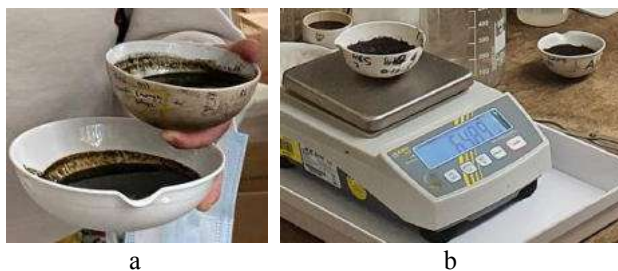
Figure 8 – Image of the digestate appearance obtained after anaerobic digestion of plant substrate and phosphogypsum: a – rare phase; b – solid phase
