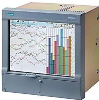
Figure 2 – Display recorder SIREC D400 [26]
