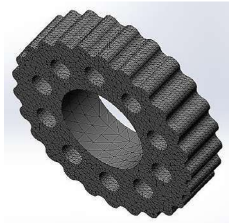
Figure 10 – Cycloid disk with FEM grid control applied
