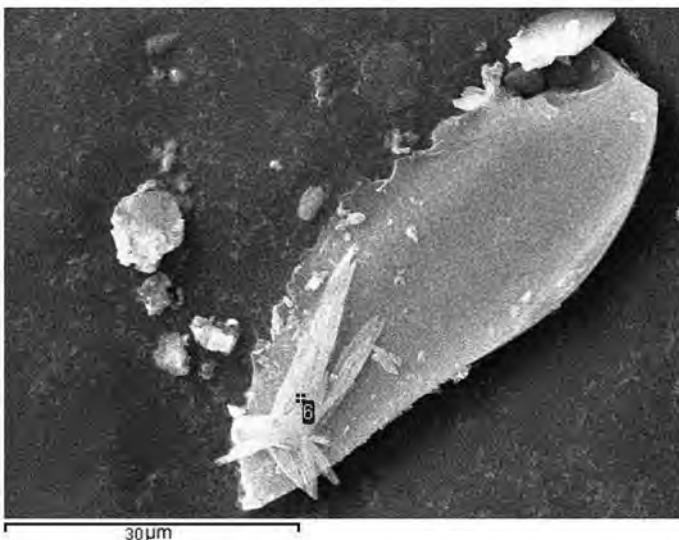
Fig. 8. Electron microscopic images of the particles and the research results of elemental composition of fragments of conglomerate coarse-shale silicate-zirconium particle (point 1) and sodium sulphide crystal sticking to it (point 3).
