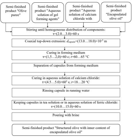
Fig. 3. Principal technological diagram of obtaining structured olive containing the encapsulated olive oil
