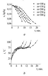
Fig. 3. Kinetics of wheat grain drying in a microwave field at different loading mass: a - change in the moisture content; b - temperature change
