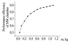
Fig. 5. Dependence of the microwave chamber's performance efficiency on the mass of water at *P*=800 W
