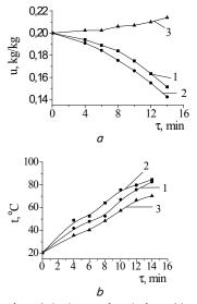
Fig. 4. Kinetics of the layer-wise drying of buckwheat in a microwave field: a - change in the moisture content; b - temperature change; 1 - upper layer; 2 - middle layer; 3 - bottom layer
