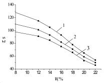
Fig. 2. Boundary curves for the wheat seed treatment time in a microwave chamber. Output power of the magnetron - 1 kW: 1 - initial temperature 10 °C;
