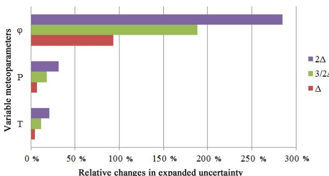
Fig. 9. Relative changes in the extended expanded uncertainty of maximum value of VCO (for the set of measurements No. 400) on the change in MSD of measuring input quantities
