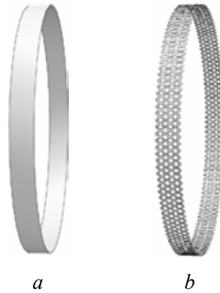
Figure 1. Estimated geometric models under consideration: a – shell model with reduced stiffness, b – perforated shell model
