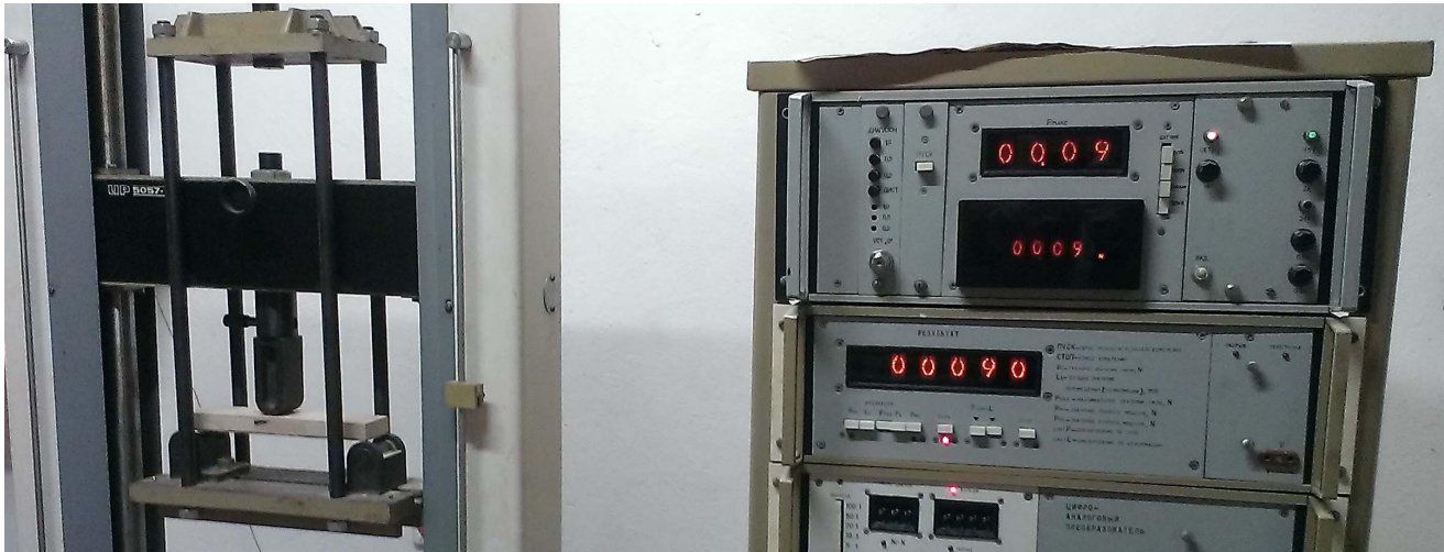
Fig. 8. Test specimen a facades blockboard with a coreboard made from PCW and face decks made from WFB at the moment of breakage
