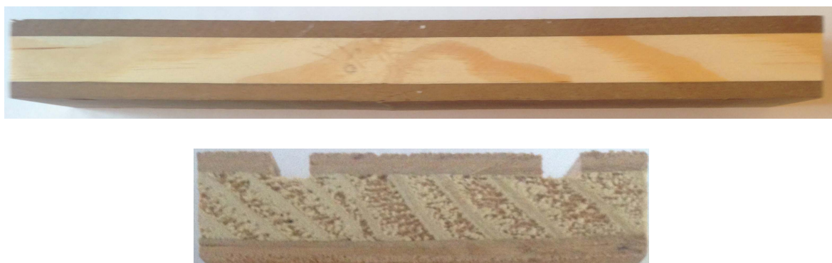
Fig. 7. Examples of front PCW-made blockboards for testing
