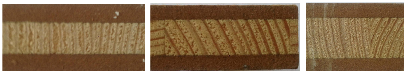
Fig. 1. Cross-section examples of front blockboards for testing
