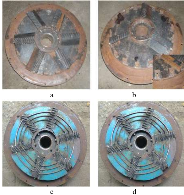
Figure 4 – Variants of execution of the stationary disk of the grating device: a – a disk with six balls fixed on it and flat plates installed in the space between the balls; b – a disk with three balls fixed on it and flat plates that, installed in the space between the balls; c – a disk with six fixed on it rings between which circular inserts with a diameter of 200, 250, and 300 mm, fixed from a rod with a diameter of 8 mm; d – a disk with 6 balls fixed on it, between which ring inserts made of a rod with a diameter of 6 mm, fixed in a circle with a diameter of 200, 250, and 300 mm
