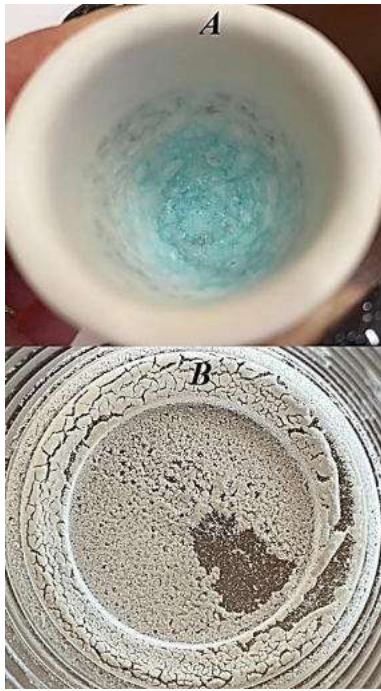
Figure 2 – Photo of the finished product of PTT after synthesis (A) and after drying (B)
