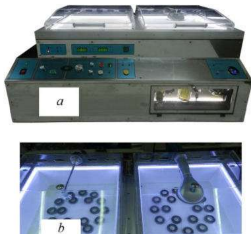
Figure 1 – Stand for pre-operational preparation of bearings: a – appearance of the stand; b – a chamber for cleaning and drying the ball bearings
