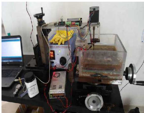
Figure 2 – Experimental setup of ECMD
