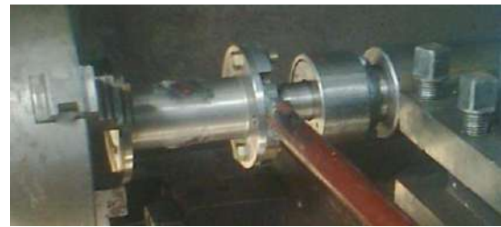
Figure 7 – Calibration of the instrument for torque measurement
