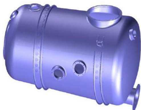
Figure 2 – Antonov-148-100 aircraft waste storage tank model
