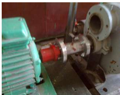
Fig. 10 – Instrument’s dynamic checks for torque measurement
