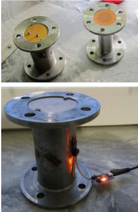
Figure 6 – Strain-gauge clutch for torque measurement
